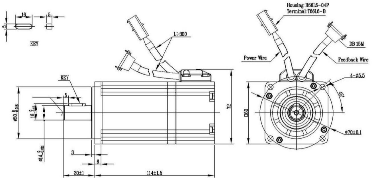
2.3.5 SMC60S-0020-30ABK-4DKH(60 法兰, 200W, 带抱闸, 增量式编码器)
